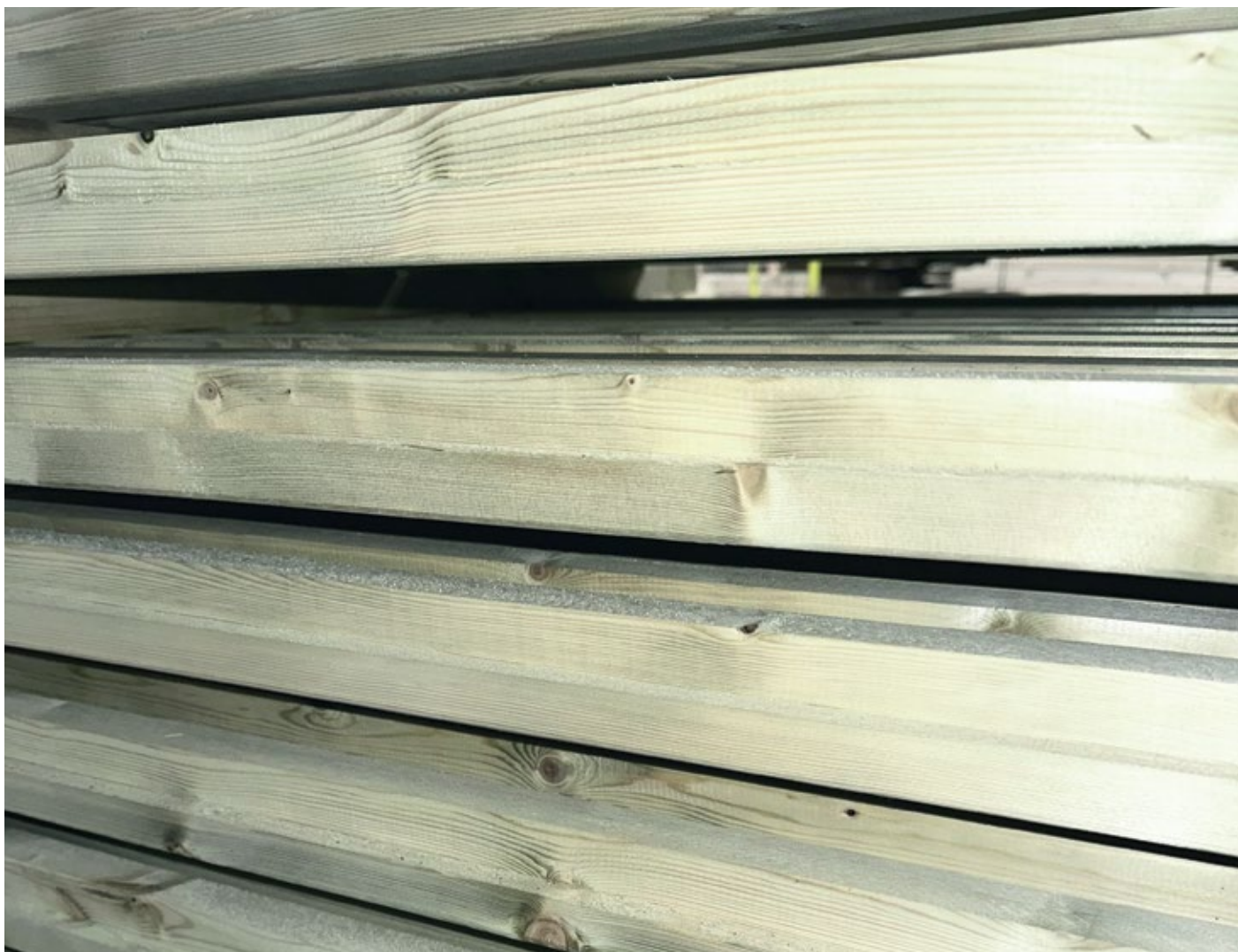
Latted timber drying process
