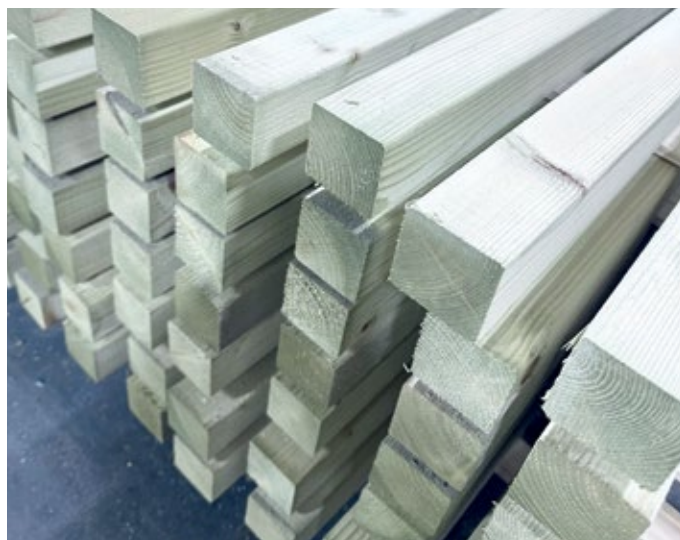
Latted timber drying process
